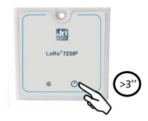
To activate the LoRa® *TEMP'* press and hold the On/Off button for more than 3 seconds. Once the device has been activated it starts measuring and transmitting data to MySirius at the set intervals.
