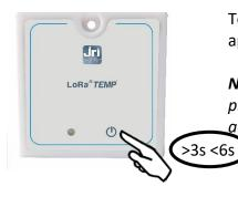
To turn off the LoRa® *TEMP'*, press and hold the On/Off button for approximately 3 to 6 seconds.
