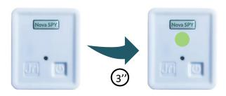
Once the battery is inserted, the device will automatically activate after 3 seconds. The NOVA SPY is self-declared in MySirius if it is within range of a Link. It starts measuring and transmitting its measurements to MySirius then flashes regularly depending on its status.
