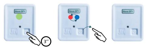
Once the device is declared in MySirius, the touch button shutdown function is disabled to prevent "accidental" switch-offs when handling the devices. It will always be possible to reactivate this option in MySirius to be able to turn off the NOVA SPY device with the touch button.
